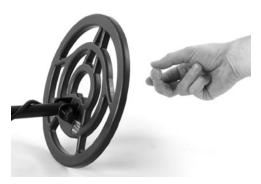
This will enable you to test typical treasure and trash items and to learn about your *GTI 2500* before taking it into the field or trying to set discrimination. Tests should be performed as shown with the searchcoil perpendicular to a bench, floor or other non-metallic surface and several feet away from any large metallic object:
