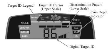
**Target ID Legend**—Works with the Target ID Cursor to indicate a target's probable identity, with Ferrous (iron) targets at the left, non-ferrous targets that are thin or have low conductivity in the middle, and thick or high conductivity targets (e.g. thick silver) at the right.
