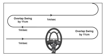
In order to fully search an area, overlap the swings of your searchcoil by half the length of the coil (about 11cm). Sweep the searchcoil in a straight line or with a slight arc at a sweep speed of about 1m/sec.
