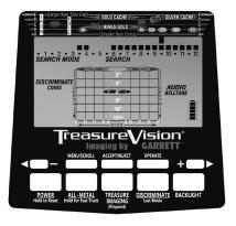
Exclusive *Treasure Imaging*<sup>TM</sup> on Garrett detectors can take the guesswork out of target identification. The LCD display above shows a quarter at about 6" depth.
