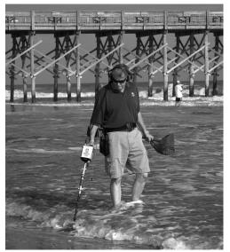
Pulse induction metal detectors such as Garrett's *Sea Hunter* and *Infinium* models ignore the mineralization effects of salt water and black sand for coin hunting at the beach.
