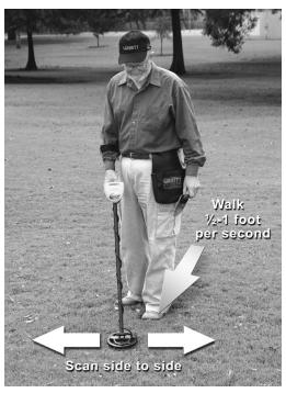
Scan side to side with the coil about 1 inch above the ground and walk 1/2 to 1 foot per second.
