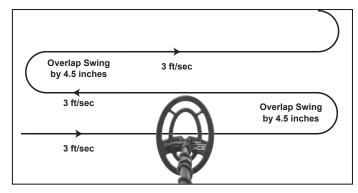
In order to fully search an area, overlap the swings of your searchcoil by half the length of the coil (about 4.5 inches). Sweep the searchcoil in a straight line or with a slight arc at a sweep speed of about 3 ft/sec.
